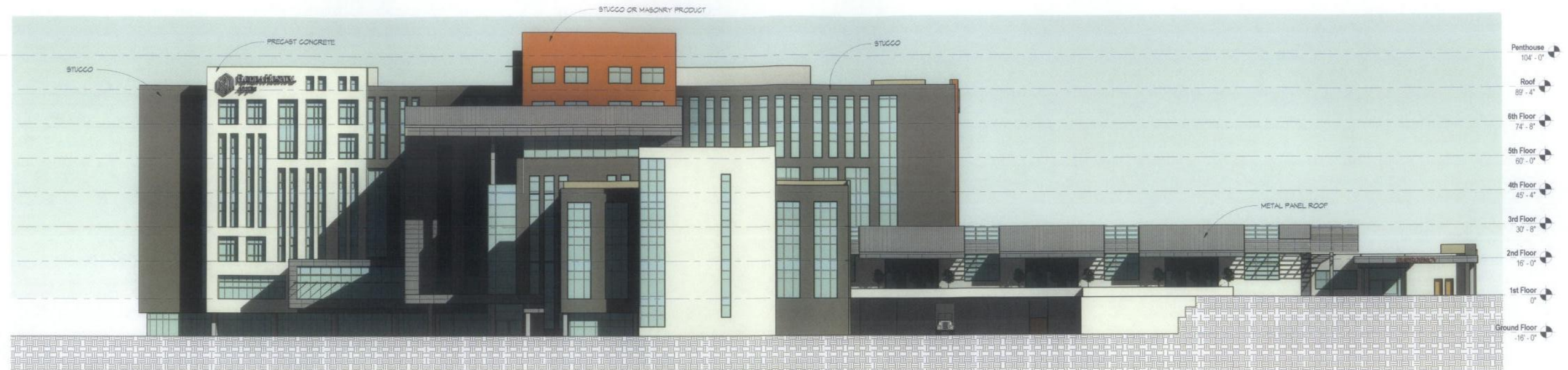
1 EAST ELEVATION SCALE: 1" = 20'-0" NOTE: PREDOMINANT MATERIALS MAY INCLUDE A MIXTURE OF PRECAST CONCRETE, STUCCO, MASONRY PRODUCTS, CAST IN PLACE CONCRETE, METAL PANELS, AND A GLASS AND ALUMINUM CURTAIN WALL SYSTEM.
