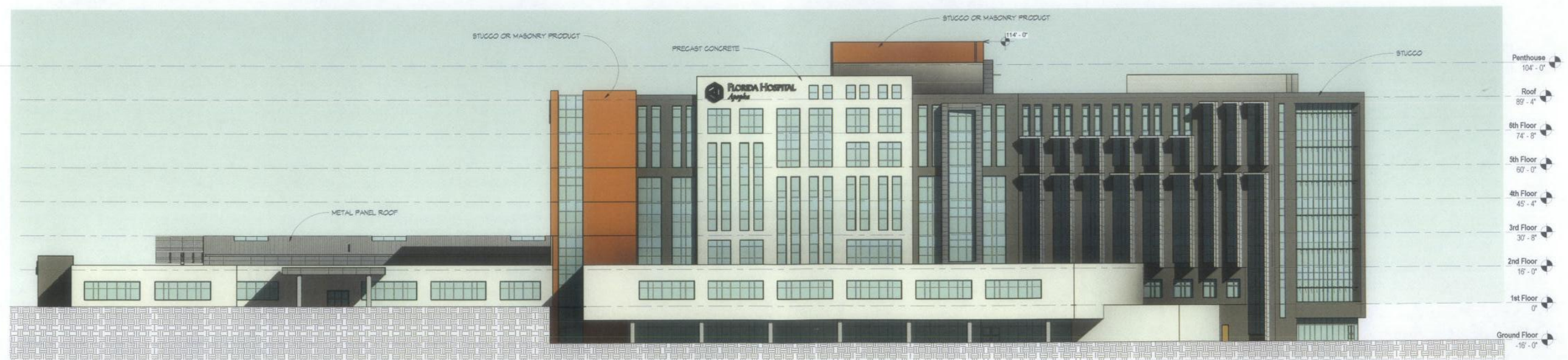
2 WEST ELEVATION SCALE: 1" = 20'-0" NOTE: PREDOMINANT MATERIALS MAY INCLUDE A MIXTURE OF PRECAST CONCRETE, STUCCO, MASONRY PRODUCTS, CAST IN PLACE CONCRETE, METAL PANELS, AND A GLASS AND ALUMINUM CURTAIN WALL SYSTEM.
